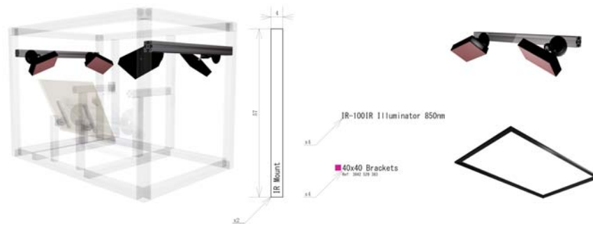
Fig. 6 Four infrared LED arrays are mounted in the table's corners, pointing downwards in order to diffuse the light and avoid overexposed areas.
