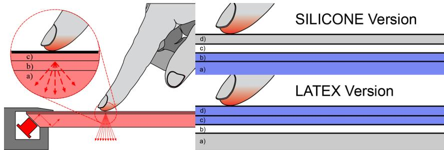
**Figure 3.** The three layers needed to track the finger touches: the polycarbonate plate (a) is covered with a compliant surface layer (b) and a diffuse layer (c) on top (left). Silicone compliant layer: the gap (c) is between the projection surface (d) and the combined silicone (b) polycarbonate (a) layer (right top). Latex compliant layer: the projection (d) and the latex layer (c) must be combined; the gap (b) is between these two and the polycarbonate plate (right bottom).
