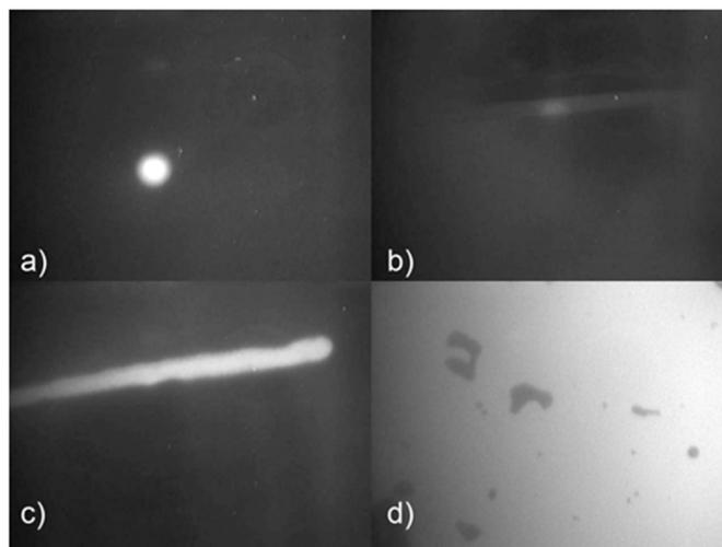
**Figure 4.** (a) Rigid PVC (backlit) (b) Rosco translucent [4] (c) Sihl polyester film 100 at, and (d) HP backlit UV. Using the wrong combination of materials can result in two main problems: (b) either the FTIR effect is not strong enough; or (d) the layers stick together.
